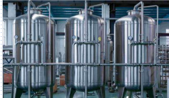
Filter system for mechanical water purification
